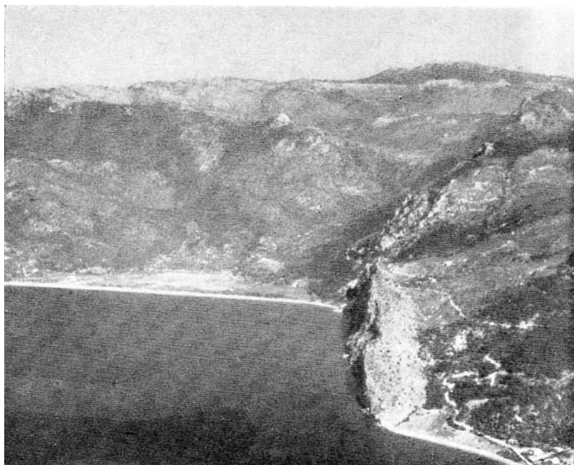
Plate 1. Oblique aerial view looking east towards the termination of the main faulting near to Psatha. The fault is nearly vertical with a throw of 250 m in the foreground. The old erosion surface in the background is not cut by an extension of the same fault. Fig. 8 is a diagrammatic interpretation of the structure.
