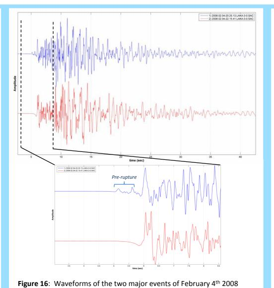
Fig. 16 shows the waveforms of the two major earthquakes of the February 4<sup>th</sup> 2008 sequence, recorded on the vertical component of the LAKA station. The full-waveform crosscorrelation maximum of the unfiltered traces is only 0.47. The waveforms have been band-pass filtered between 1-20Hz, however this results to a lower  $XC_{max}$  value of 0.35. By correlating only the P-waves,  $XC_{max}$  rises only up to 0.38, while the waveforms are aligned as shown in the close-up.
