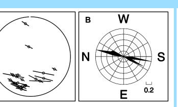
Figure 13: (A) Polar equal-area projections on the upper hemisphere of the fast shear wave polarizations at LAKA station. The length of the bars is proportional to the time delay of each event and the circle represents an angle of incidence equal to 45°. (B) Rose diagram of the fast shear wave polarization directions at LAKA station.
