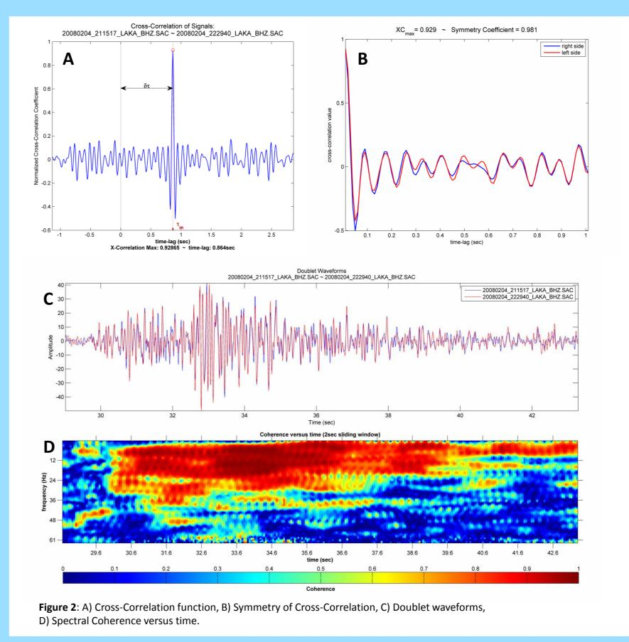
The LAKA station, installed by the University of Athens, is located about 15km N of this earthquake swarm. The relatively small distance of this station permits the detection of many microearthquakes within the swarm, most of which occur in small volumes and consist multiplet clusters. Such microearthquakes have similar seismic parameters and thus produce similar waveforms when recorded at a station on the surface.
